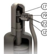
Palanca estanca Sealed packing lever
